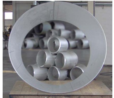
20" sch. 140 Elbow according to UNS S31254 (SMO)
